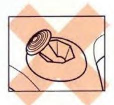
If the Control Stick is held at an angled position (as shown in the picture on the left) when the power is turned ON, this position will be set as neutral. This will cause games using the Control Stick to operate incorrectly.
